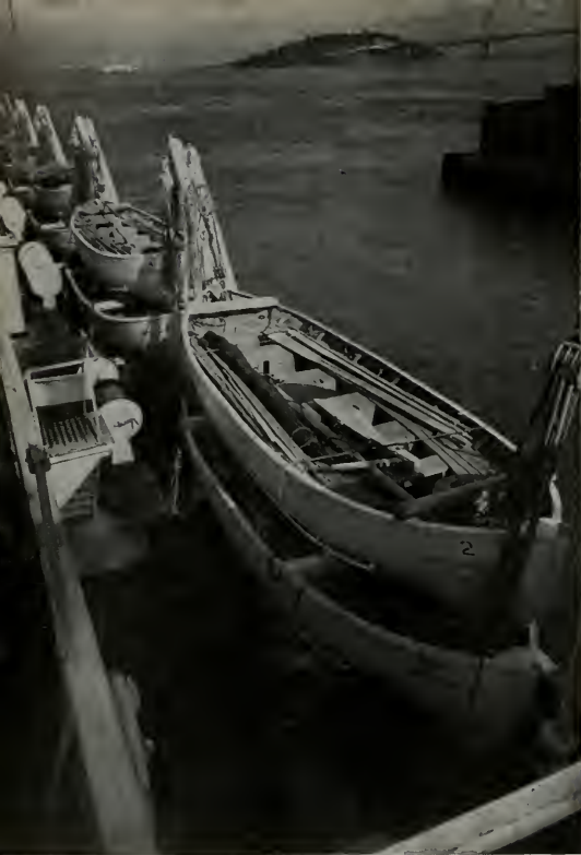
A row of Welin nested lifeboats and boom type davits with boat gear complete.
